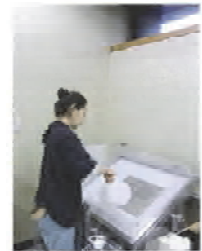
6. Repair process using a leaf casting machine
